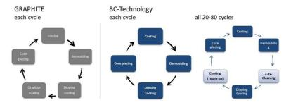
It is only after a great number of castings, that any interventions are necessary with the BC technology. The time needed for these interventions is similar to the one needed for graphite application – which is required for every single run.
